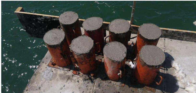
**PROBERAS DE CONCRETO F'C= 350KG/CM2 DE CONCRETO IN SITU**
